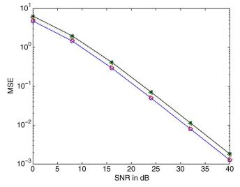
Fig. 2. MMSE using the true channel (" $-\circ$ "), expectation of the MSEs for channel inaccuracies only at transmitter (" $\triangleright$ "), expectation of the MSEs for channel inaccuracies only at the receiver (" $\triangleleft$ ") and expectation of the MSEs for channel inaccuracies at both the transmitter and the receiver (" $-\ast$ ").
